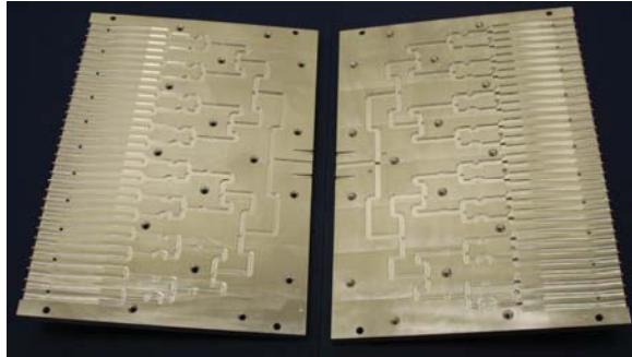
Fig. 17. Fabricated 76-GHz array.
