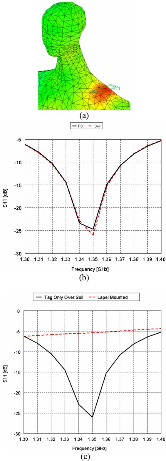
Fig. 7. Body worn antenna (a) in-situ model, (b)  $S_{11}$  when in free space (black) compared to soil (red) and (c) over soil with (red) and without (black) the body.
