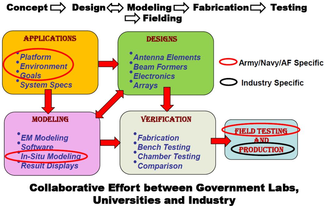
Fig. 1. Components of antenna development for military applications.
