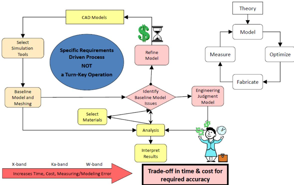
Fig. 2. Modeling flow-chart for electromagnetic simulation.
