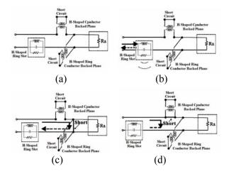
Fig. 8. (a) The conceptual equivalent-circuit model for the proposed antenna, (b) for the new resonance frequency, (c) for the first notched frequency, and (d) for the second notched frequency.
