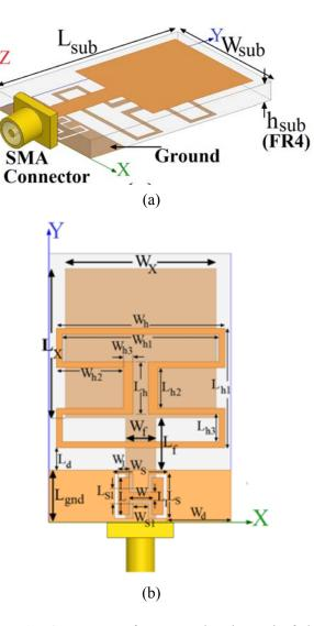
Fig. 1. Geometry of proposed microstrip-fed monopole antenna, (a) side view, (b) bottom view.
