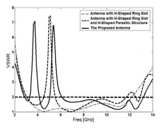
Fig. 6. Simulated VSWR characteristics for the various antenna structures shown in Fig. 5.
