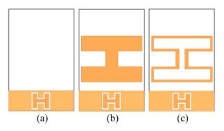
Fig. 5. (a) The basic structure (ordinary square monopole antenna with an H-ring slot in the ground plane), (b) basic structure with an H-shaped conductor backed plane, and (c) basic structure with an H-ring conductor backed plane.
