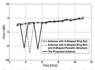
Fig. 11. Maximum gain comparisons for the basic structure (simulated), basic structure with H-shaped parasitic structure (simulated), and the proposed antenna (measured).
