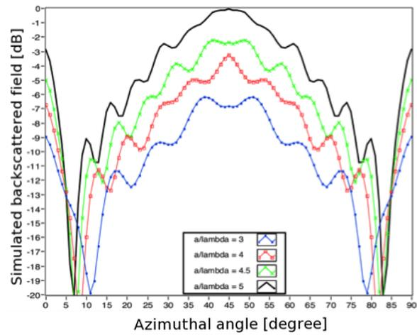
Fig. 1. Simulated dihedral backscattering for different dihedral dimensions. The graph shows the backscattered field (in dB) versus the azimuthal angle (0, 90°). The blue curve is relative to  $a/\lambda = 3$ ; the red curve is relative to  $a/\lambda = 4$ ; the green curve is relative to  $a/\lambda = 4.5$ ; finally, the black curve is relative to  $a/\lambda = 5$ . The different curves are separated of 6, 4, 2 dB, respectively, from the black one.
