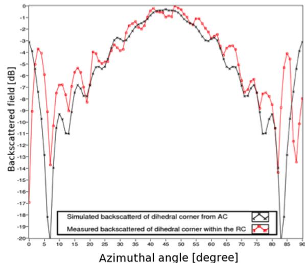
Fig. 3. Comparison between the backscattering measurement from the dihedral corner with  $a/\lambda = 5$  performed within the RC (red line) and the simulated one (black line), versus the azimuthal angle.
