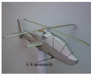
(a) Scale model helicopter (10:1 scale)
