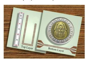
Fig. 13. The fabricated prototype of the proposed high Q-factor BSF.
