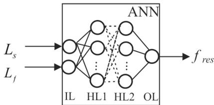
Fig. 3. ANN model of RF MEMS switch resonant frequency.
