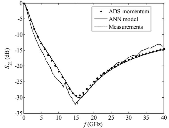
Fig. 8. Isolation of the fabricated RF MEMS switch ( $L_s = 174 \mu\text{m}$  and  $L_f = 40 \mu\text{m}$ ).
