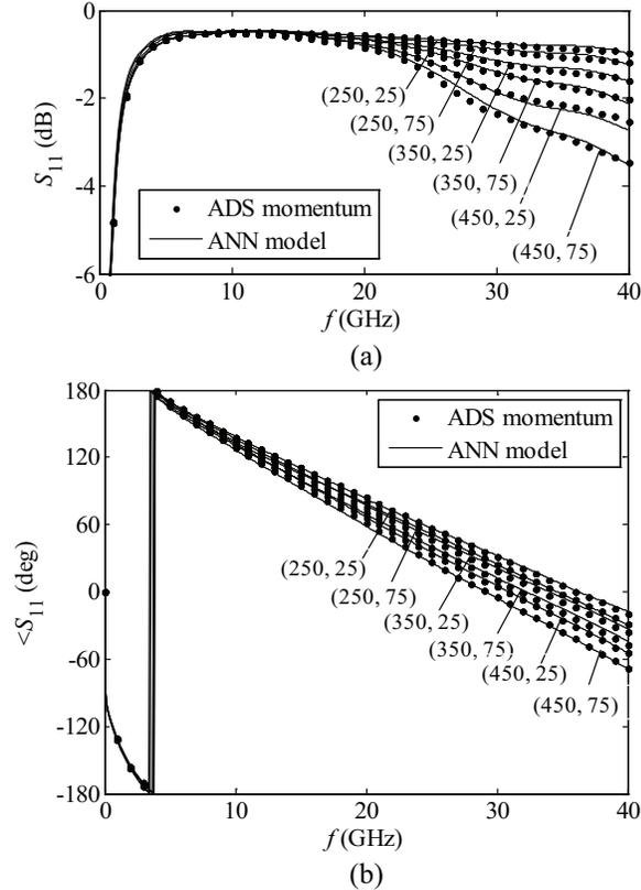
Fig. 6. Parameter  $S_{11}$  for six ( $L_s$  [ $\mu\text{m}$ ],  $L_f$  [ $\mu\text{m}$ ]) combinations not used for the model development: (a) magnitude and (b) phase.
