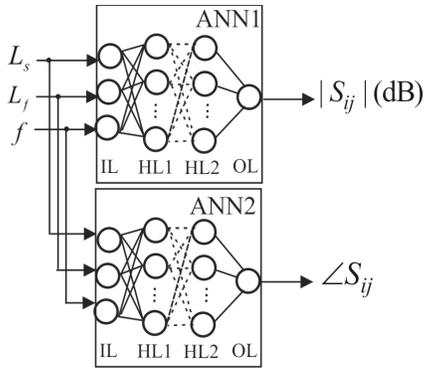
Fig. 2. ANN model of RF MEMS switch S-parameters.
