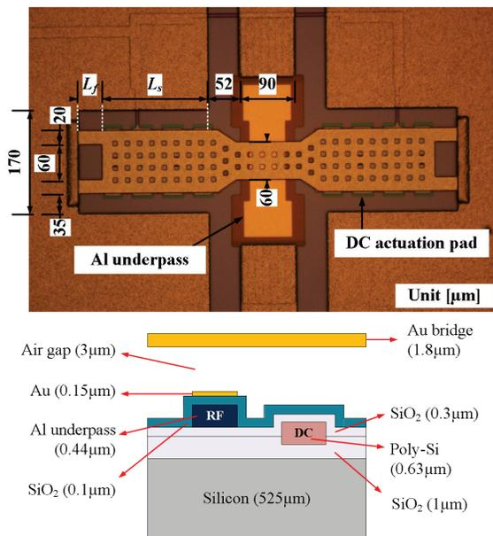
Fig. 1. Top-view of the realized RF MEMS switch and schematic of the cross-section with 8 layers in FBK technology [12].
