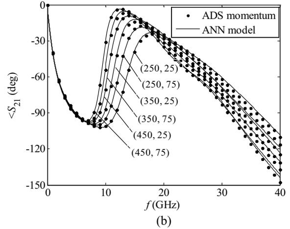
Fig. 7. Parameter  $S_{21}$  for six ( $L_s$  [ $\mu\text{m}$ ],  $L_f$  [ $\mu\text{m}$ ]) combinations not used for the model development: (a) magnitude and (b) phase.
