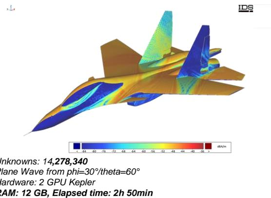
Fig. 3. Equivalent electric current on a Sukhoi, induced by an impinging plane wave @ 10 GHz, evaluated by using a fast IPO formulation.
