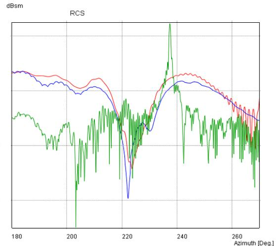
Fig. 5. VV monostatic scattered field of the intake in Fig. 4, modelled with thin walls (red) and with the proposed method (blue). The platform contribution (green) is also shown.
