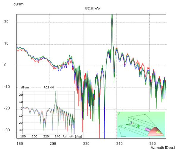
Fig. 6. VV monostatic scattered field of the UCAV in Fig. 4, considering the complete structure (blue), or combining separate contribution from the intake and the platform (red). Inclusion of a small part of the fuselage (inset) in solving the intake allows to obtain a more accurate result (green). Similar results are obtained for the HH polarization (inset).
