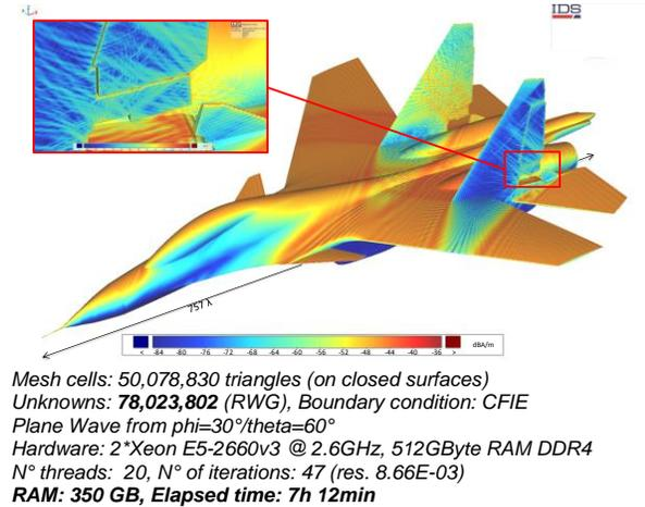
Fig. 1. Equivalent electric current on a Sukhoi, induced by an impinging plane wave @ 10 GHz.
