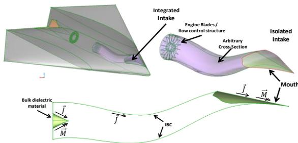
Fig. 4. Typical Air intake isolated problem.
