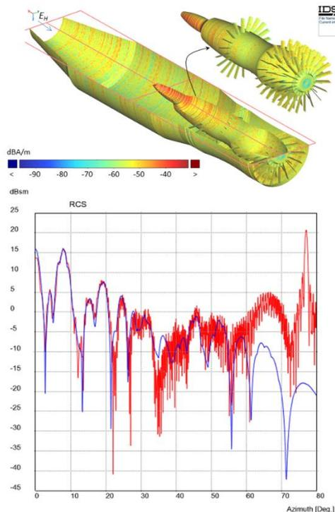
Fig. 7. Equivalent electric current (top) and monostatic Scattered field (bottom) for a  $5.17 \text{ m} \times 1.19 \text{ m} \times 1.19 \text{ m}$  Intake @ 10 GHz (10,824,636 unknowns and CFIE+IBC formulation), modelled with thin walls (red) and with the proposed method (blue).
