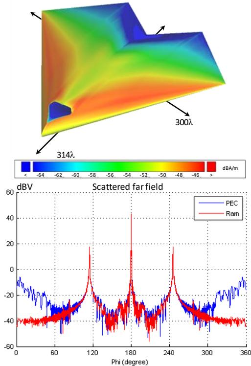
Fig. 2. Equivalent electric current (top) and scattered field (bottom) for a UCAV, induced by an impinging plane wave @ 10 GHz. Pec labels refers to an intake without a RAM covering.
