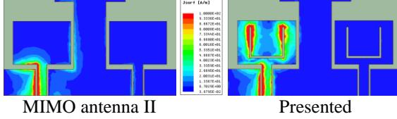
Fig. 5. Surface current distributions of the MIMO antenna II and the proposed MIMO antenna at 5.5 GHz.
