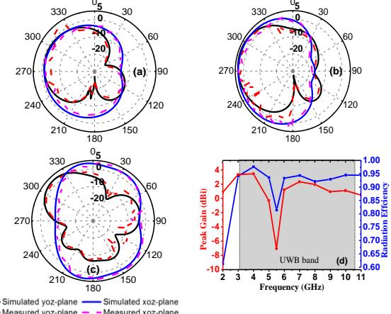
Fig. 7. Simulated and measured radiation pattern of UWB MIMO antenna at: (a) 4 GHz, (b) 7 GHz, (c) 10 GHz, and (d) measured peak gain and radiation efficiency of the proposed UWB MIMO antenna.
