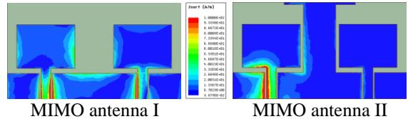
Fig. 3. Surface current distributions of MIMO antenna I and MIMO antenna II at 4.6 GHz.
