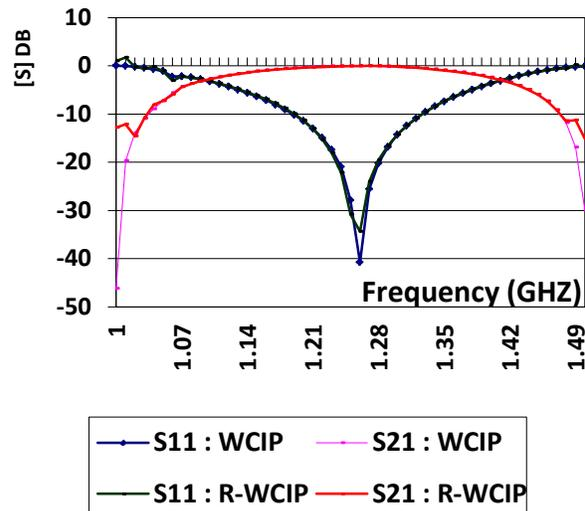
Fig. 10. Parameter “S” in function of frequency, 50 basic iterations before reducing the matrices dimensions,  $N_{max}=200$  iterations, contour vicinity with step=3.
