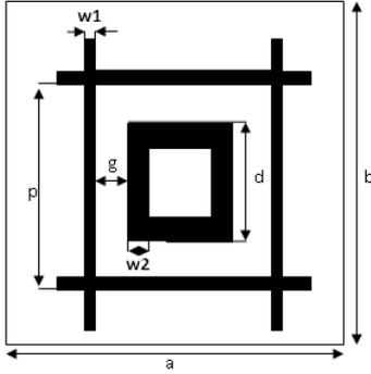
Fig. 1. Unit cell of a FSS structure.
