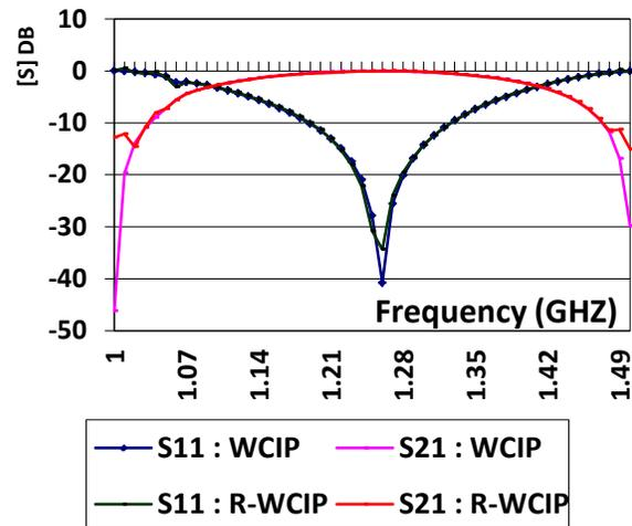
Fig. 9. Parameter “S” in function of frequency, 50 basic iterations before reducing the dimensions of the matrices,  $N_{max}=200$  iterations, contour vicinity with step=1.
