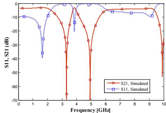
Fig. 8. The simulated results of  $S_{11}$ ,  $S_{21}$  for 2<sup>nd</sup> and 3<sup>rd</sup> harmonics suppression mode.
