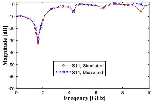
Fig. 5. Measured and simulated input return loss of power divider for the 3<sup>rd</sup> and 5<sup>th</sup> harmonics suppression mode.
