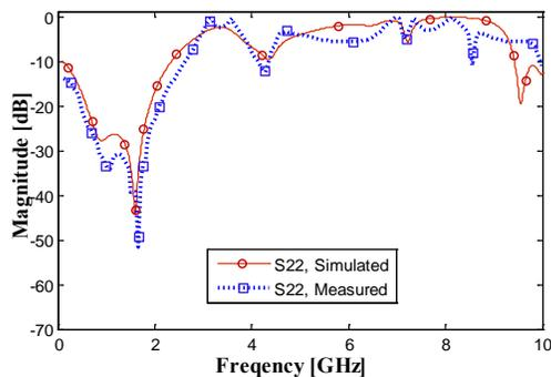
Fig. 6. Measured and simulated output return loss of power divider for 3<sup>rd</sup> and 5<sup>th</sup> harmonics suppression mode.
