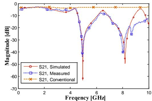
Fig. 4. Measured and simulated insertion loss of power divider for the 3<sup>rd</sup> and 5<sup>th</sup> harmonics suppression mode.
