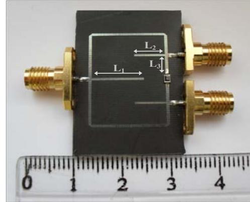
Fig. 3. Photograph of the fabricated power divider.
