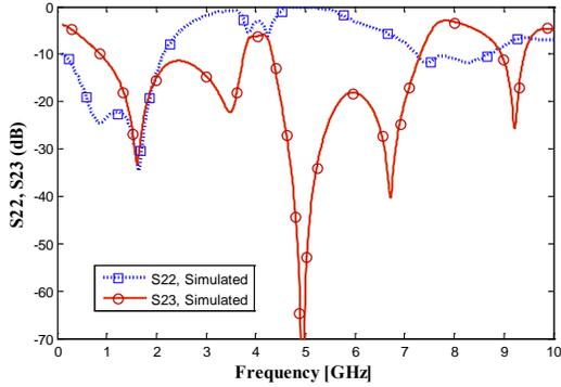
Fig. 9. Simulated results of  $S_{22}$  and  $S_{23}$  for 2<sup>nd</sup> and 3<sup>rd</sup> harmonic suppression modes.
