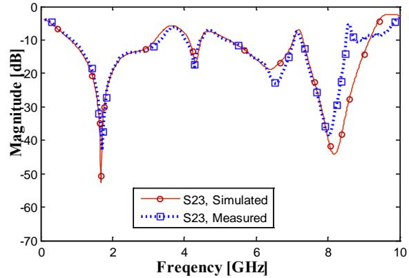
Fig. 7. Measured and simulated isolation of power divider for 3<sup>rd</sup> and 5<sup>th</sup> harmonics suppression mode.
