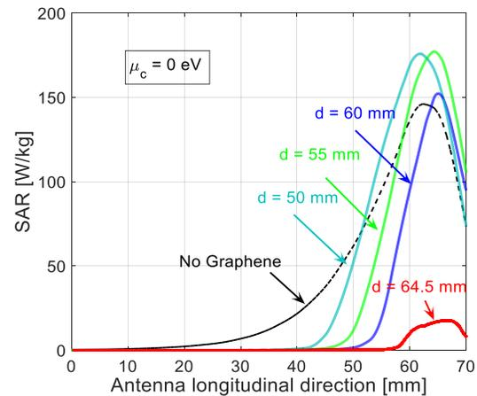
Fig. 8. Specific Absorption Rate (SAR) along the antenna at 1.5 mm from the outer conductor for the 2<sup>nd</sup> configuration for different distances between graphene and the slot. The feedline is at 0 mm and the slot is located at 65 mm.
