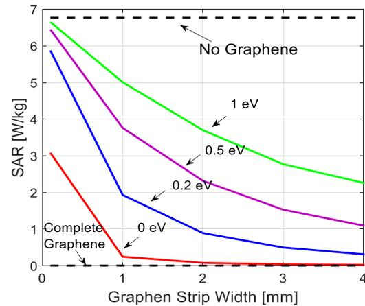
Fig. 9. SAR at 30 mm from the feedline vs. the width  $w$  of the graphene strip, for different level of chemical potential.
