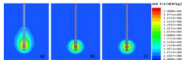
Fig. 10. SAR on a plane parallel to the axis of the antenna: (a) the reference antenna, (b) 2<sup>nd</sup> configuration (Fig. 4 (b)), 3<sup>rd</sup> configuration (Fig. 4(c)).
