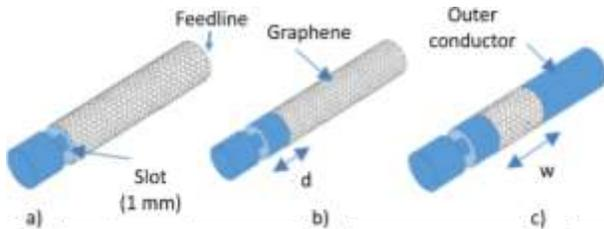
Fig. 4. Microwave coaxial antenna with the graphene sheet: (a) antenna fully covered by the graphene sheet from the slot all the way to the feedline; (b) graphene shifted from the slot and covering all the way to the feedline; (c) graphene strip shifted from the slot.
