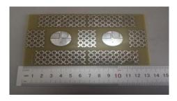
Fig. 13. Photographs of the fabricated EBG antenna.
