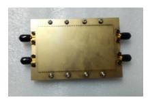
Fig. 10. The photograph of the SISL coupler.
