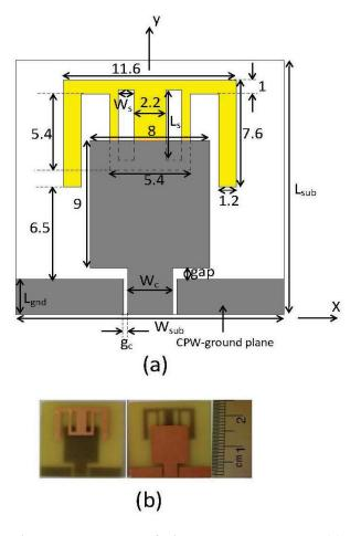
Fig. 1. Geometry of the propose antenna: (a) dimensions (units: mm) and (b) photograph of fabricated antenna.
