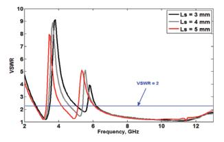
Fig. 4. Simulated band-rejection of the proposed antenna for various values L<sub>s</sub>.
