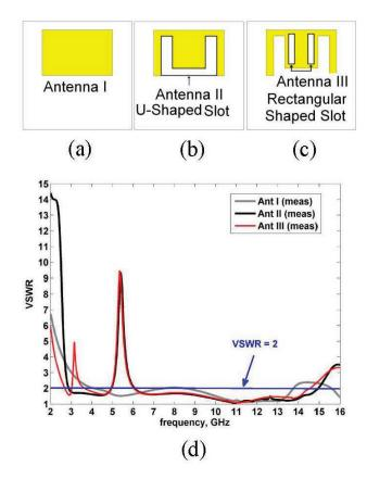
Fig. 5. Geometry of conductor-backed plane: (a) ordinary conductor-backed plane, (b) with U-shaped slot, (c) with a pair of mirror rectangular-shaped slots and (d) measured VSWR characteristics for a, b and c.
