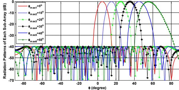
Fig. 3. The far field patterns of each sub-array of the 6x20 rectangular planar antenna using the Dolph-Chebyshev amplitudes given in Table 3.
