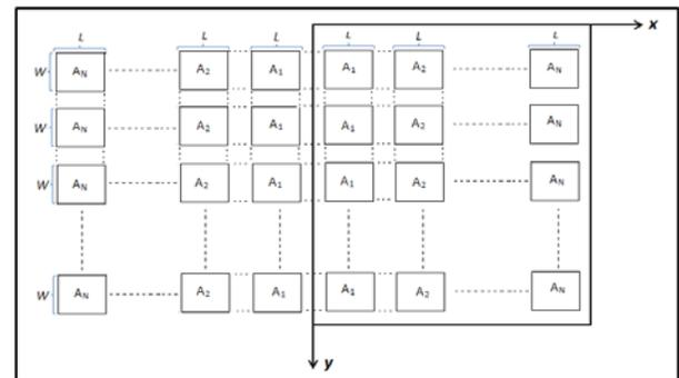
Fig. 5. A rectangular planar patch antenna array.
