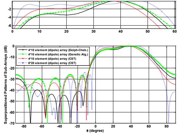
Fig. 4. The Dolph-Chebyshev and optimized far field patterns of the 4x10 element planar array, and the CST simulations of the 4x10 element and 6x20 element planar arrays.
