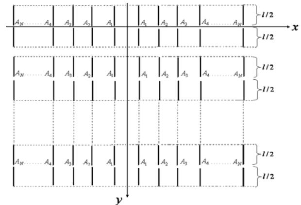
Fig. 1. A rectangular planar half-wave dipole antenna array.
