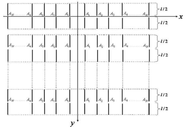
Fig. 1. A rectangular planar half-wave dipole antenna array.
