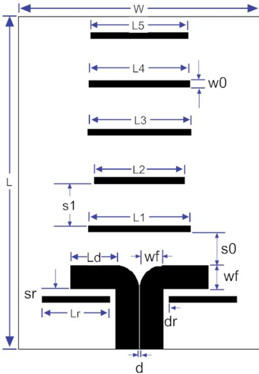
Fig. 1. Schematic diagram of the proposed quasi-Yagi antenna.
