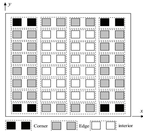
Fig. 10. Combined-elements in a 2-D  $(8 \times 8)$ -element array.
