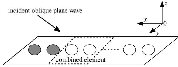
Fig. 3. Combined-element in a 1-D finite array.
