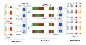
Fig. 3. The parallelization of matrix-vector multiplication for  $Z_{far}I$ .
