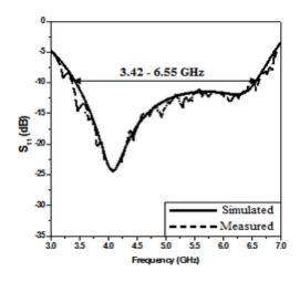
Fig. 6. Simulated and measured return losses.
