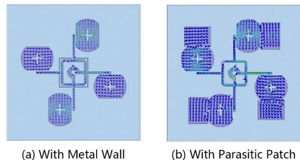
Fig. 9. Simulated current distributions at  $0^\circ$ , 5.87GHz: (a) with metal wall and (b) with parasitic patch.
