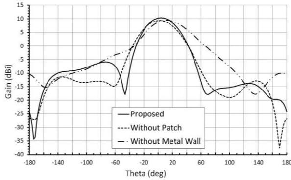
Fig. 10. Pattern comparisons of the proposed antenna at 5.87GHz (xoz-plane).
