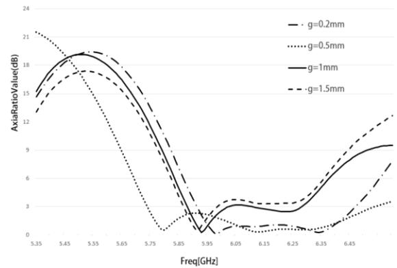
Fig. 3. Simulated AR of the  $2 \times 2$  array with different  $g$ .
