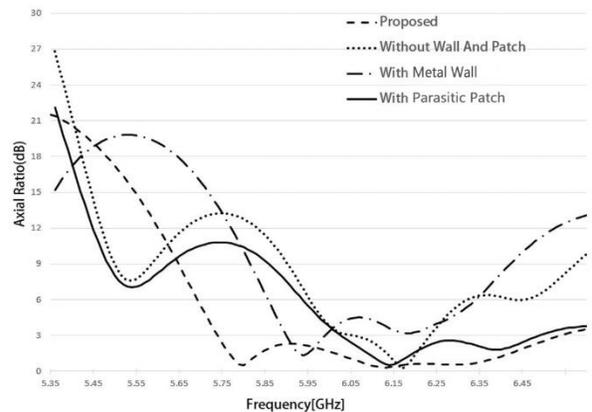
Fig. 5. Simulated AR of the  $2 \times 2$  array.
