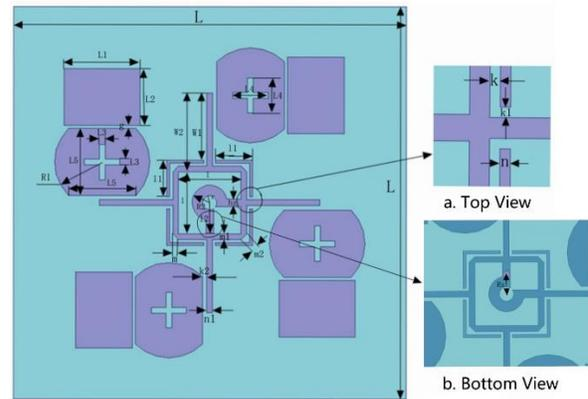
Fig. 1. Geometry and dimensions of the proposed antenna array.
