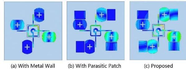
Fig. 7. Simulated vector electric field distributions at  $0^\circ$ , 5.87GHz: (a) with metal wall, (b) with parasitic patch, and (c) proposed.
