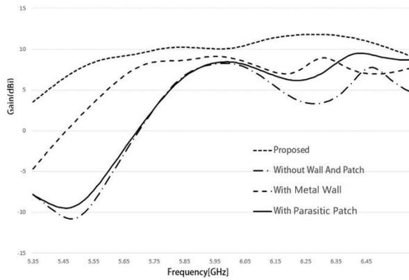
Fig. 6. Simulated gains of the  $2 \times 2$  array.
