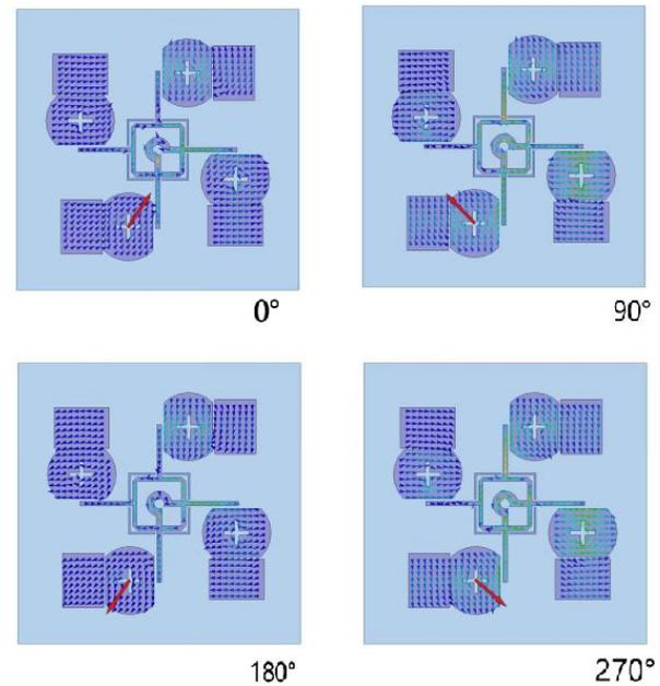
Fig. 8. Simulated current distributions at 5.87GHz.
