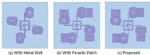
Fig. 2. Stages of antenna development: (a) with metal wall, (b) with parasitic patch, and (c) proposed antenna.
