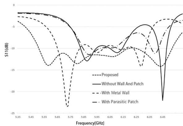
Fig. 4. Simulated return loss of the  $2 \times 2$  array.
