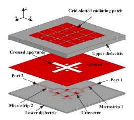
Fig. 1. Perspective view of the proposed dual-polarized grid-slotted microstrip antenna.
