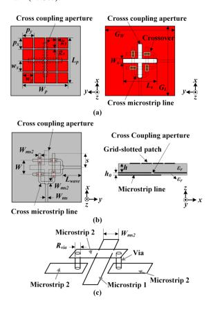
Fig. 2. Geometry of the proposed grid-slotted microstrip antenna: (a) top view of the radiating patch and GND, (b) bottom view of the feeding structure and side view of the overall structure, and (c) stereograph of the crossover.
