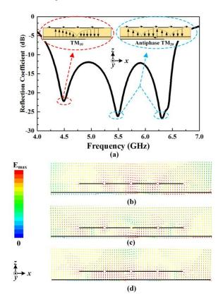
Fig. 5. Simulated reflection coefficient and E-field distribution of the proposed antenna. (a) Simulated reflection coefficient and sketches of the resonant modes. The vector electric field distributions at (b) 4.5 GHz, (c) 5.5 GHz, and (d) 6.3 GHz.
