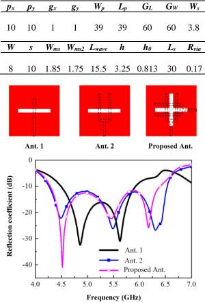
Fig. 3. Design evolution and simulated reflection coefficients.
