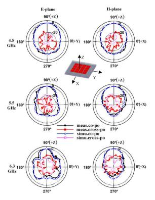
Fig. 8. Simulated and measured normalized radiating patterns at port 2 of the Proposed Ant. at 4.5 GHz, 5.5 GHz and 6.3 GHz.
