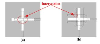
Fig. 4. Cross feeding structure: (a) with two orthogonal straight microstrip lines, and (b) with two orthogonal Y-shaped microstrip lines.
