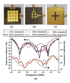
Fig. 6. Photographs and measured results of the fabricated Proposed Ant. (a) Top view, (b) bottom view, (c) the ground plane and cross coupling apertures in the GND layer, and (d) simulated and measured reflection and transmission coefficients.
