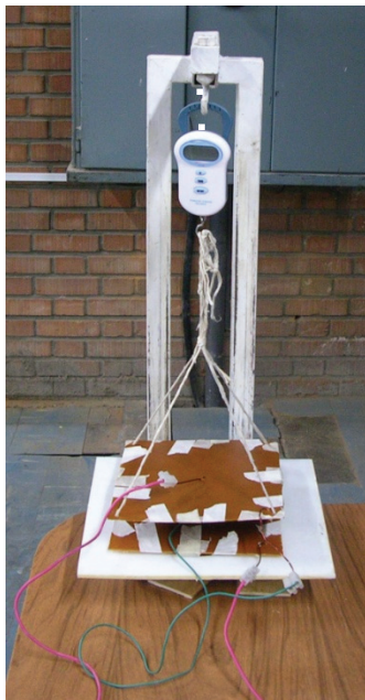
Fig. 7. Measurement of the magnetic force between the two spiral coils.
