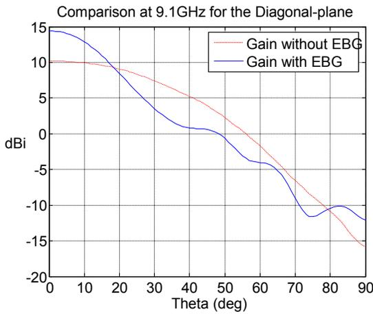
Fig. 14. Comparison for the antenna gain in the diagonal-plane cut with and without grids.
