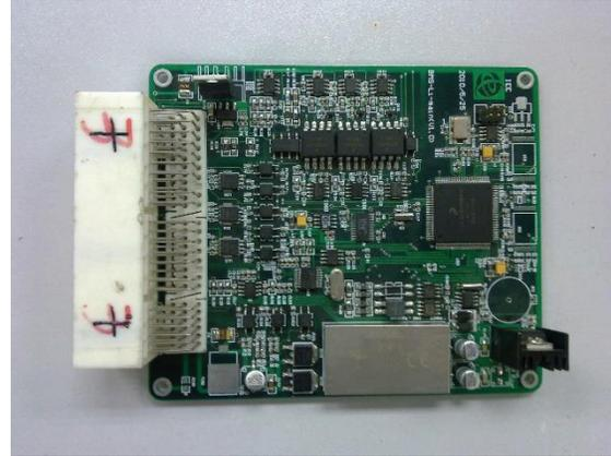
Fig. 8. Photo of the battery management system.
