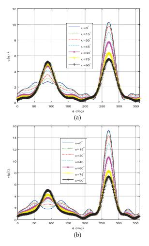
Fig. 4. Normalized bistatic width versus scattering angle for PEMC elliptic cylinders of different admittances coated with  $\varepsilon_{rc}=2.5$ ,  $\mu_{rc}=1.0$ ,  $\phi_i=90^\circ$ : (a)  $\zeta_c=0.002$ , and (b)  $\zeta_c=0.0015$ .
