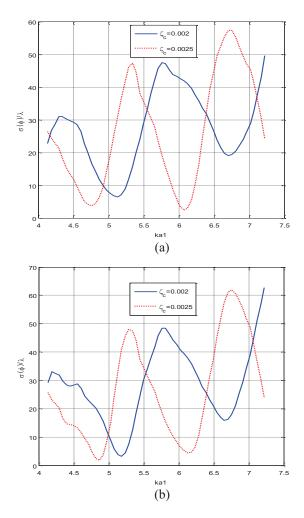
Fig. 6. Normalized bistatic width versus ka<sub>1</sub> for PEMC elliptic cylinders of different admittances coated with  $\epsilon_{\rm rc}$ =3.0,  $\mu_{\rm rc}$ =1.0,  $\phi_i$ =0.0°, *a*=0.4 $\lambda$ , *b*=0.2 $\lambda$ : (a) v=45°, and (b) v=75°.
