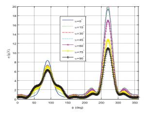
Fig. 5. Normalized bistatic width versus scattering angle for PEMC elliptic cylinders of different admittances coated with  $\varepsilon_{\rm rc}$ =3.0,  $\mu_{\rm rc}$ =1.0,  $\phi_i$ =90° and  $\zeta_c$ =0.002.
