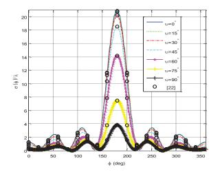
Fig. 2. Normalized bistatic width versus scattering angle for PEMC elliptic cylinders of different admittances coated with  $\varepsilon_{\rm rc}$ =2.5,  $\mu_{\rm rc}$ =1.0,  $\phi_i$ =0°, and  $\zeta_c$ =0.0.
