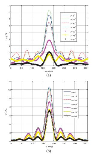
Fig. 3. Normalized bistatic width versus scattering angle for PEMC elliptic cylinders of different admittances coated with  $\varepsilon_{\rm rc}$ =2.5,  $\mu_{\rm rc}$ =1.0,  $\phi_i = 0^{\circ}$ : (a)  $\zeta_c = 0.002$ , and (b)  $\zeta_c = 0.0015$ .
