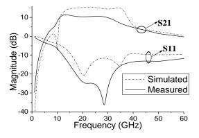
Fig. 2. Simulated (in dash line) and measured S-parameters (in solid line).
