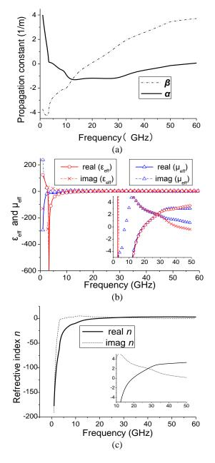
Fig. 3. (a) Extracted complex propagation constant  $\gamma(\alpha+j\beta)$  from measured two-port S-parameter. (b) Extracted effective permittivity  $\varepsilon_{eff}$  (red) and effective permeability  $\mu_{eff}$  (blue) from measured two-port S-parameter. The inset shows the details near zero-Y-axis. (c) Extracted index of refraction *n* from measured two-port S-parameter. The inset shows the details near zero-Y-axis.
