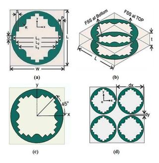
Fig. 1. FSS unit cell structure: (a) top view, (b) perspective view, (c) unit cell rotation at  $45^{\circ}$ , and (d) A 2 × 2 unit cell array.
