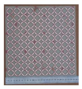
Fig. 8. Photograph of the fabricated FSS prototype.
