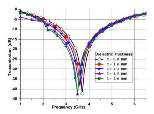
Fig. 7. Resonat frequency variations with respect to dielectric thickness.
