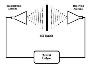
Fig. 9. FSS free-space measurement method.
