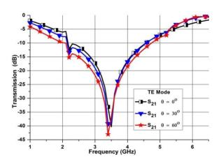
Fig. 5. Transmission response of FSS element rotated at 45° for TE mode.
