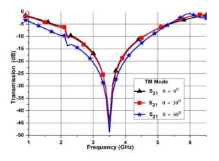
Fig. 4. S<sub>21</sub> plot for TM mode over oblique angle variations.
