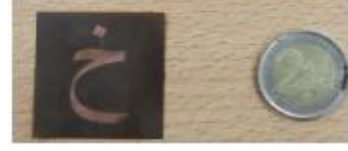
Fig. 5. Photograph of the chipless tag based on the connected Arab letter "خ".
