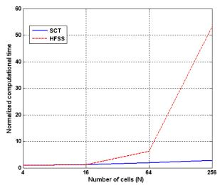
Fig. 12. Evolution of computing time compared to the standard time for the calculation of two cells of uniform arrays on the same computer.
