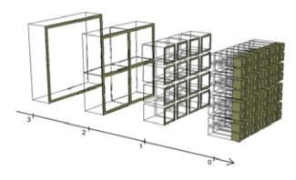
Fig. 2. An example of partitioning of finite size and thick dichroïc metallic mirror.
