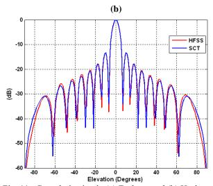
Fig. 11. Co-polarization in (a) E-plane, and (b) H-plane @ 15 GHz.
