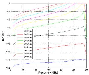
Fig. 9. Design dimension sweep of the aperture length L of 16 x 16-element uniform thick dichroïc plate.
