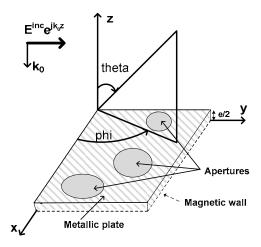
Fig. 6. Scattering problem in free space in the conventional coordinates system [14].
