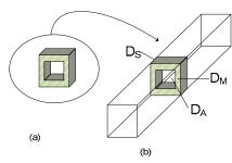
Fig. 4. (a) Initial lossless metallic pattern with a passive sub-domain DS presenting many fine geometrical details; (b) artificial rectangular waveguide of cross section DS in which the set of propagating and evanescent modes constitutes the basis for the electromagnetic field.
