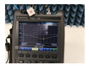
Fig. 5. Experimental measurements of  $S_{11}$  for the circularly polarized patch antenna using vector network analyzer of the Agilent Field Fox N9918A.
