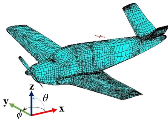
Fig. 2. Cross-dipole onboard Beechcraft Bonanza WIPL-D model.
