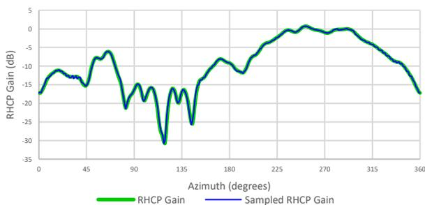
Fig. 4. Gain comparison of discrete sampling to reference case.
