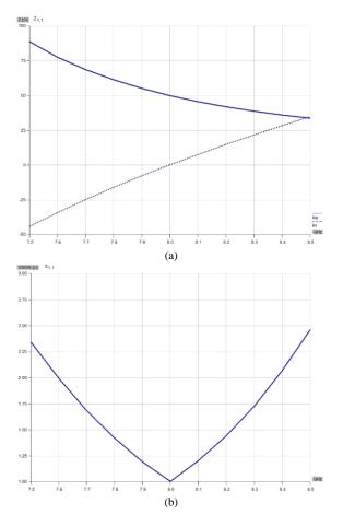
Fig. 2. Slot antenna parameters: (a) input impedance; (b) VSWR.
