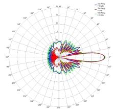
Fig. 4. Slot array principal azimuth cut overlays.
