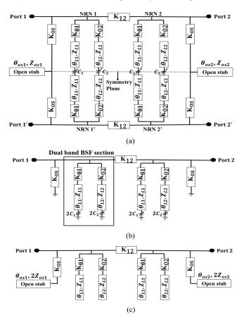
Fig. 1. (a) Schematic of the proposed topology, (b) DM equivalent circuit, and (c) CM equivalent circuit.
