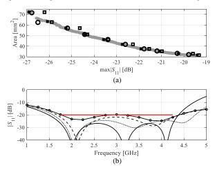
Fig. 3. (a) Pareto-optimal solutions: (o) initial set obtained with MOEA, (\*) selected designs for refinement, (□) EM-simulated selected designs, (O) EM-simulated refined designs; (b) reflection characteristics of the transformer for selected Pareto-optimal designs.
