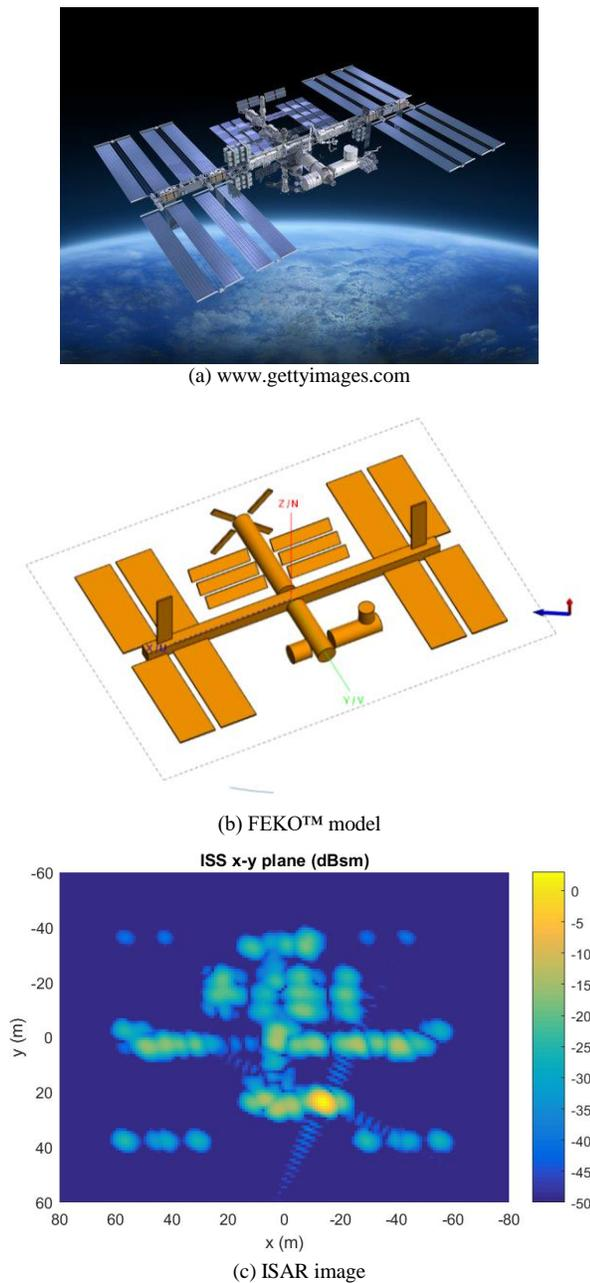
Fig. 2. International Space Station (ISS). (a) ISS in orbit. (b) FEKO model. (c) UHF ISAR image projected in the  $x$ - $y$  plane seen from an elevation slant plane of  $10^\circ$  (dBsm). A  $10^\circ$  azimuth window is used to generate the image.
