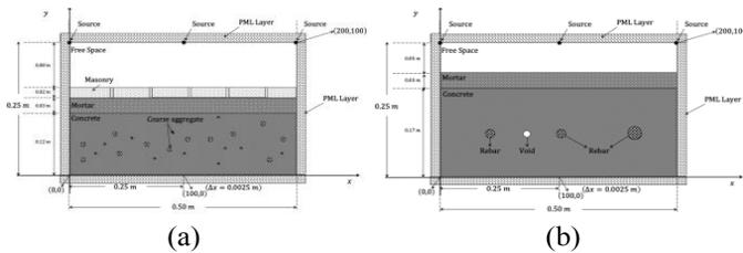
Fig. 2. Numerical model of computation domain: (a) Case A; (b) Case B.
