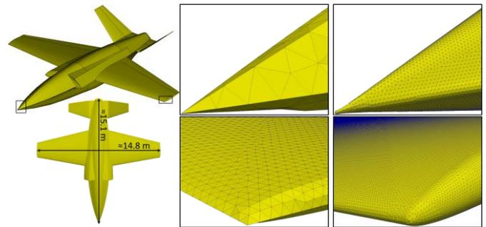
Fig. 1. The surface of the EXPEDITE-RCS model visualized from the defeatured IGS file (left) and triangular meshes of the model's nose and wingtip using an average edge length of  $\sim 2$  in (middle) and  $\sim 0.25$  in (right).
