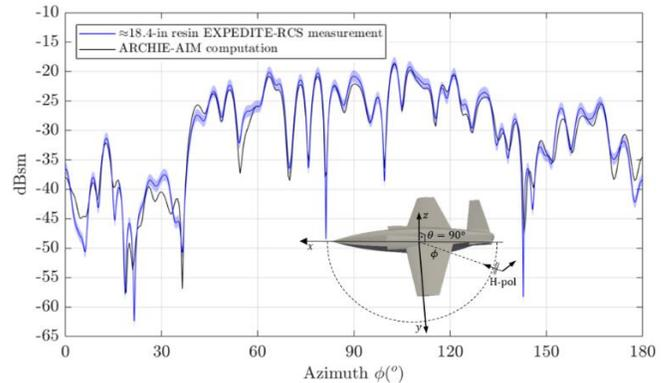
Fig. 3. Measured and computed HH-polarized monostatic RCS at 7 GHz for the  $\sim 18.4$ -in long uncoated-resin model. The measured data are shown with a  $\pm 1$  dB uncertainty band [10]. The computed data were generated using the resin material properties in [11].
