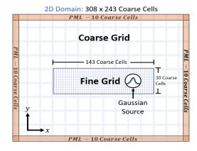
Fig. 1. Example from [1, Section 7.5.2]: Line source simulated with a 2D FDTD code. Striped box respresents physical location of fine grid region.
