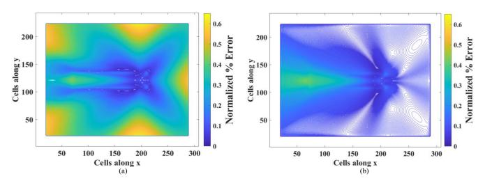
Fig. 2. Normalized percentage errors for the 2D FDTD as described in Fig. 1 and Table I for 1:3 contrast ratio: (a) S22 errors and (b) HS24 errors.
