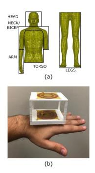
Fig. 2. (a) ANSYS human body model, and (b) 10mm measurement setup on the hand.
