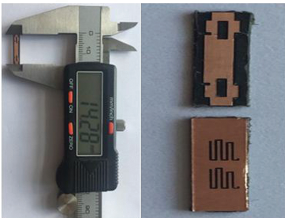
Fig. 14. Photograph of the manufactured DMS-DGS BSF.
