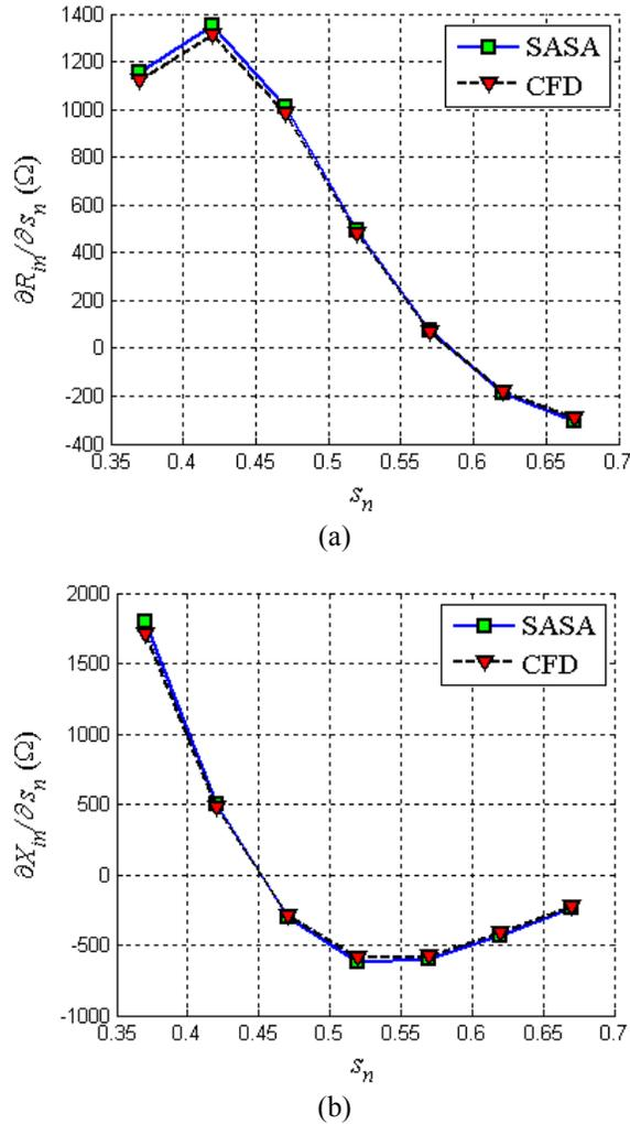
Fig. 4. Sensitivity of the input impedance of the Yagi-Uda antenna with respect to the distance between the driving element and the reflector: (a) resistance derivative; (b) reactance derivative.
