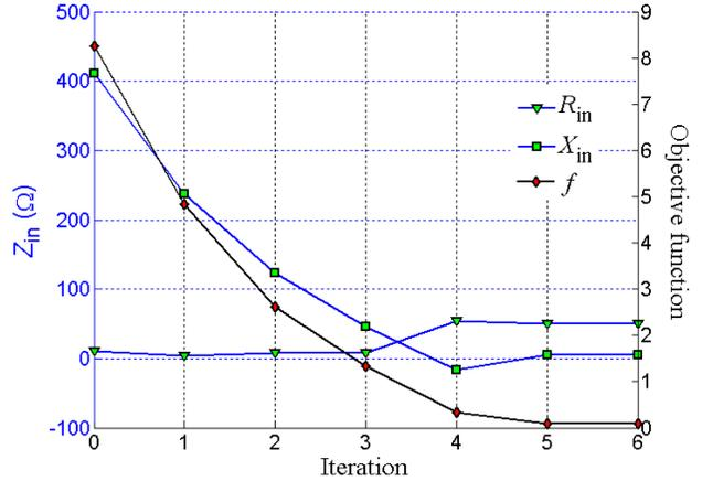
Fig. 9. Progress of the objective function and the input impedance during the optimization without sensitivity information.
