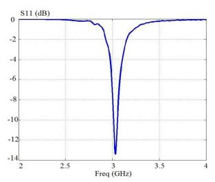
Fig. 3. S11 for patch antenna above the biased ferrite substrate.
