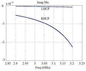
Fig. 7. Real and imaginary parts of effective permeability for RHCP and LHCP.
