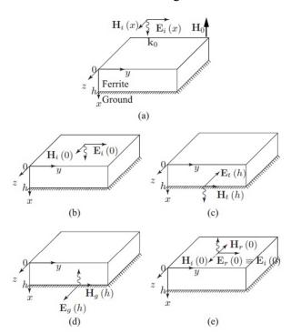
Fig. 1. (a to e) show the way that how a grounded ferrite can propose a PMC condition on its surface [11].
