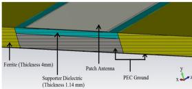
Fig. 2. The perspective view and side cut view of patch antenna on the ferrite substrate.
