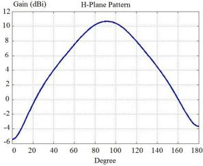
Fig. 4. Directivity of improved patch, E-plane and H-plane at  $f_0$ = 3.03GHz.
