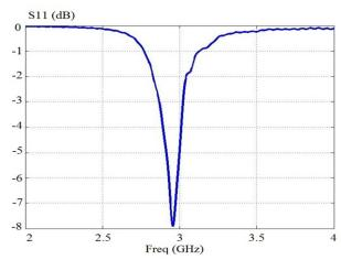
Fig. 5. The upper figure is the schematic of dipole antenna above the grounded biased ferrite substrate and the lower figure is the S11 of the antenna.
