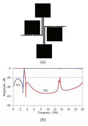
Fig. 10. The new structure (a) layout and (b) simulation results.
