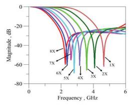
Fig. 6. The response of the proposed resonator for different scale factors.
