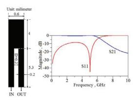
Fig. 1. Conventional hairpin resonator and its S-parameters results.
