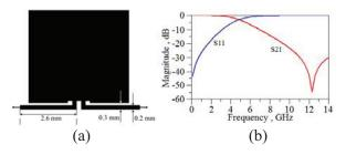
Fig. 9. The second modified Hairpin unit (a) the structure and (b) simulation results.
