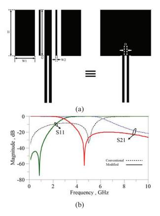
Fig. 3. (a) Modified hairpin resonator and (b) comparison between the results of the conventional and modified hairpin resonator.
