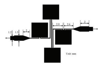
Fig. 11. The proposed lowpass filter.
