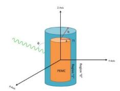
Fig. 1. PEMC Cylinder coated with topological insulator.
