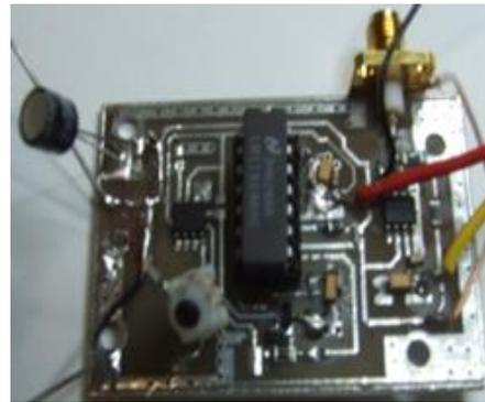
Fig. 13. Manufactured envelope amplifier circuit.
