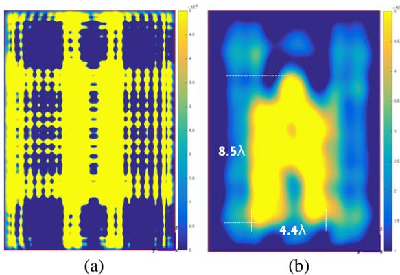
Fig. 10. Image reconstructed from: (a) the corrupted signal and (b) the cross-correlated data.
