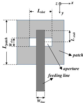
Fig. 2. Geometry of the primary feed (bottom view).
