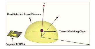
Fig. 4. Measurement configuration of the hemi-spherical phantom.
