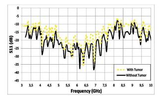
Fig. 9. S<sub>11</sub> results for deeply buried tumor (at X<sub>1</sub> point).
