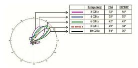
Fig. 2. Beam variation of the antenna proposed in [17].
