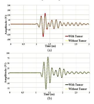
Fig. 11. Reflected time domain signals: (a) antenna is at the closest, and (b) antenna is at the farthest to the tumor.
