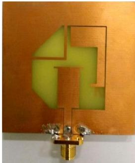
Fig. 2. Photograph of the fabricated antenna.
