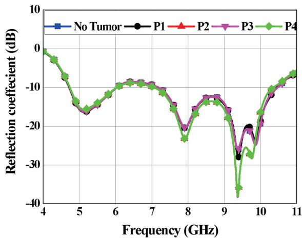
Fig. 20. The reflection coefficients  $S_{44}$  for all cases.
