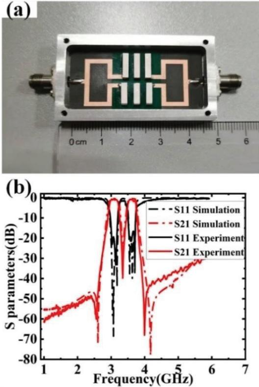
Fig. 5. (a) The fabricated DBPF. (b) Simulated and measured S-parameters.
