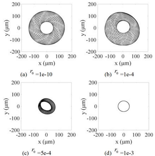
Fig. 28. Rotor orbit at 46 Hz for different  $r_0$ .
