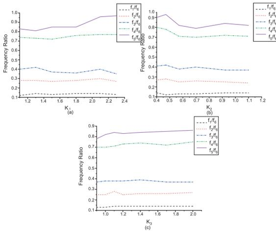
Fig. 3. Frequency characteristics of the proposed quad-section SIRs with varied admittance ratios.
