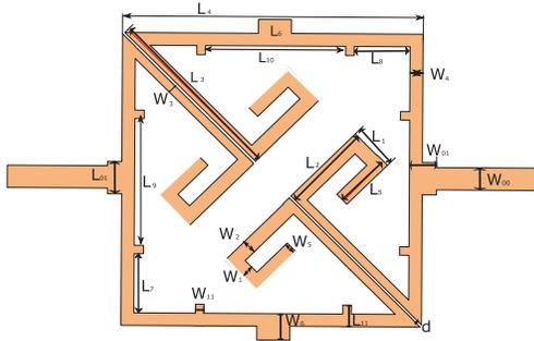
Fig. 6. Layout of designed sext-band BPF.
