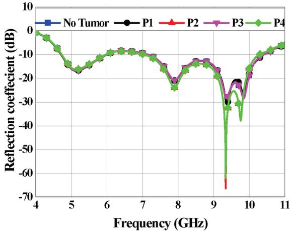
Fig. 18. The reflection coefficients  $S_{22}$  for all cases.
