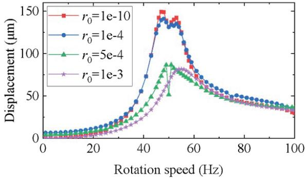
Fig. 24. Displacement response during run-up for different  $r_0$ .
