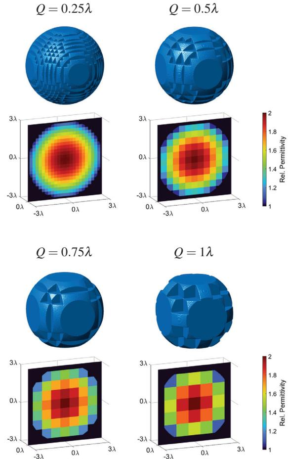
Fig. 3. Visualizations of macro cell LL as the cell edge length  $Q$ , is varied from  $0.25\lambda$  to  $1\lambda$ . Radius of lens is held constant at  $3\lambda$ . Below each 3D model is a 2D slice through the center of the lens and colorized to reveal the relative permittivity distribution.
