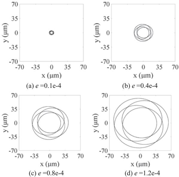
Fig. 9. Rotor orbit at 80 Hz for different  $e$ .
