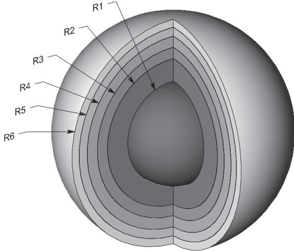
Fig. 9. Example of a multiple layer spherical LL with wedge cut out to expose interior construction. The central core has radius  $R1$ , and the five surrounding shells have outer radii of  $R2$  through  $R6$ .
