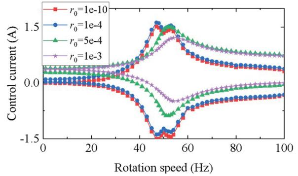
Fig. 26. Control current response for different  $r_0$ .
