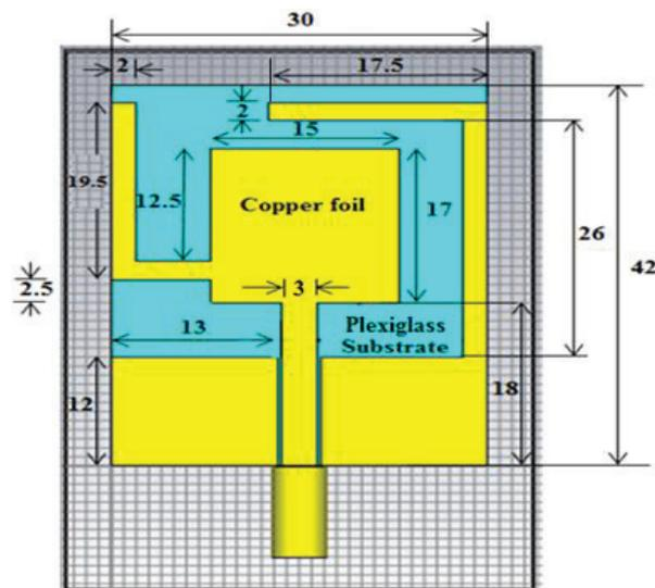
Fig. 1. Geometry and dimensions of the proposed antenna.
