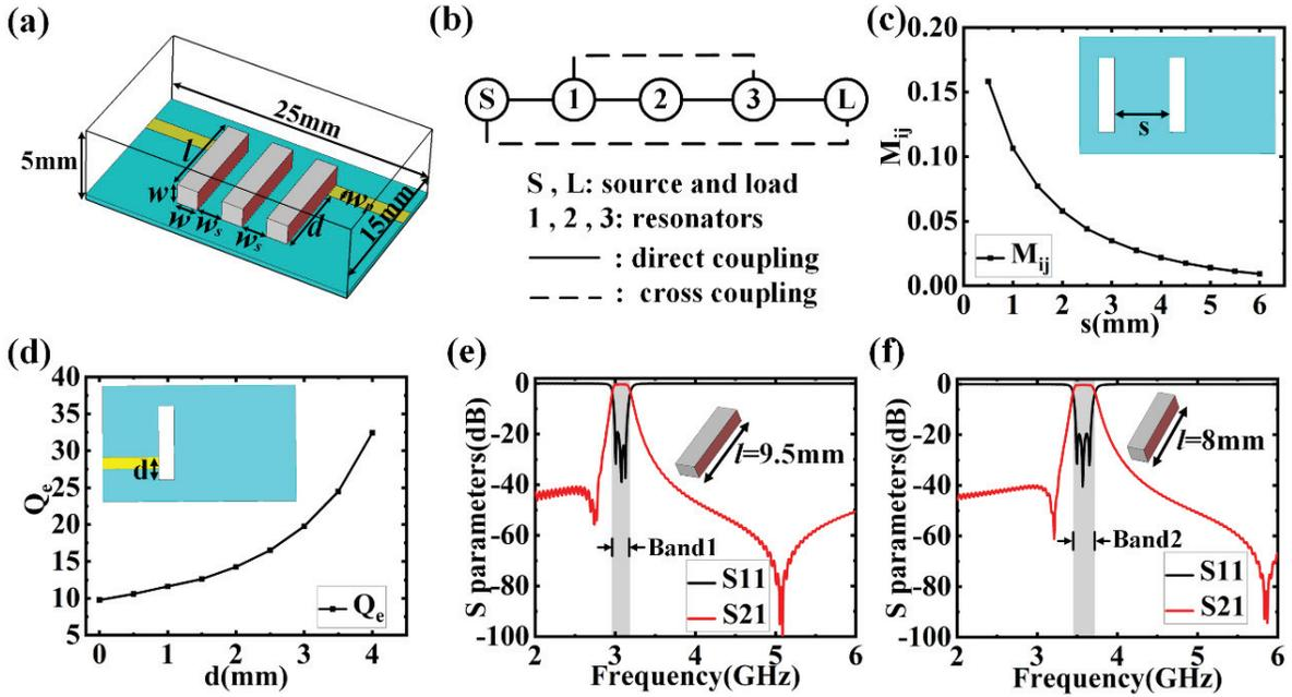
Fig. 3. A Single BPF based on  $\frac{\lambda_g}{4}$  planar ELSPR. (a) Schematic diagram of the BPF. (b) Coupling routes. (c) Coupling coefficient between two adjacent ELSPRs. (d) The calculated  $Q_e$  of the BPF. (e) and (f) S-parameters of filter I and II with passband Band 1 and Band 2 respectively.
