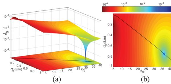
Fig. 8. Estimation of soil parameters for the bare land region named “Bare Land 2”. Plots of the function  $\delta_S$  given by (20) versus the real dielectric constant  $\epsilon_{rg}$  and conductivity  $\sigma_g$  of a clayey soil; (a) 3D, (b) 2D, plot.
