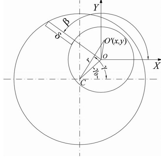
Fig. 2. Schematic diagram of motor's air gap with mixed eccentricity.
