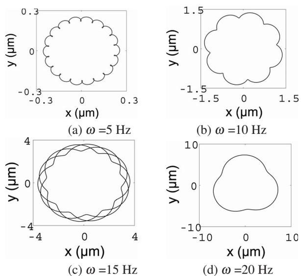
Fig. 3. Rotor orbit for different rotation speeds.
