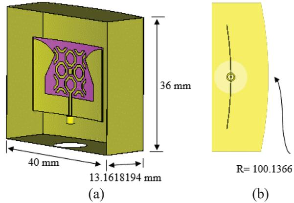
Fig. 10. (a) The front side of the cavity structure. (b) The top side of the cavity structure.
