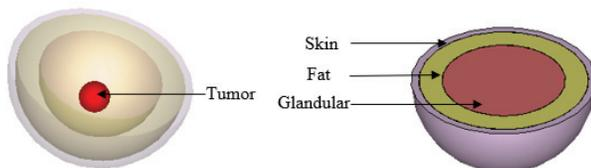
Fig. 14. Different layers of the proposed heterogeneous phantom.
