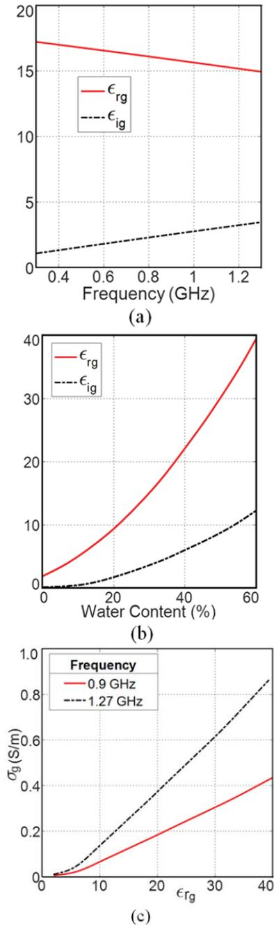
Fig. 2. Dependence of the complex relative permittivity of the clayey soil on the frequency and volumetric water content. (a) Dispersive properties at 30% water content, (b) Dependence of  $\epsilon_{rg}$  and  $\sigma_g$  on the water content, (c)  $\epsilon$ - $\sigma$  characteristic curves.
