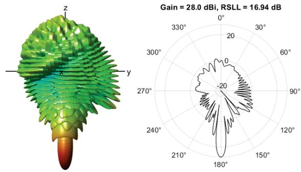
Fig. 15. The RSLL is determined by examining individual 2D cuts through the full 3D radiation pattern. Cuts are taken every  $5^\circ$  and are sampled with a  $\theta$  resolution of  $0.25^\circ$ . This pattern is for the lens ( $Q = 1\lambda, r_l = 5\lambda$ ) with feed location of  $(\theta_a = 78.75^\circ, \phi = 22.5^\circ)$ .
