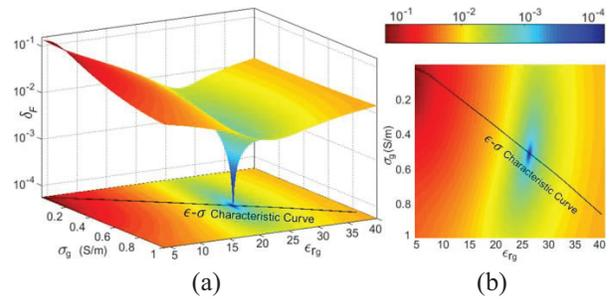
Fig. 6. Estimation of soil parameters for the forest region named “Forest 3”. Plots of the quantity  $\delta_F$  given by (10) versus the real dielectric constant  $\epsilon_{rg}$  and conductivity  $\sigma_g$  of a clayey soil; (a) 3D, (b) 2D, plot.
