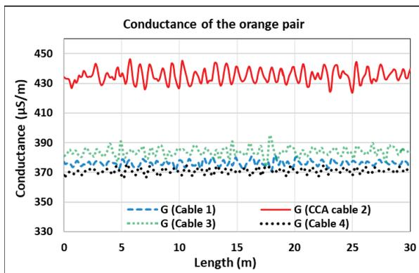
Fig. 8. Conductance comparison of the four cables using the orange pair.
