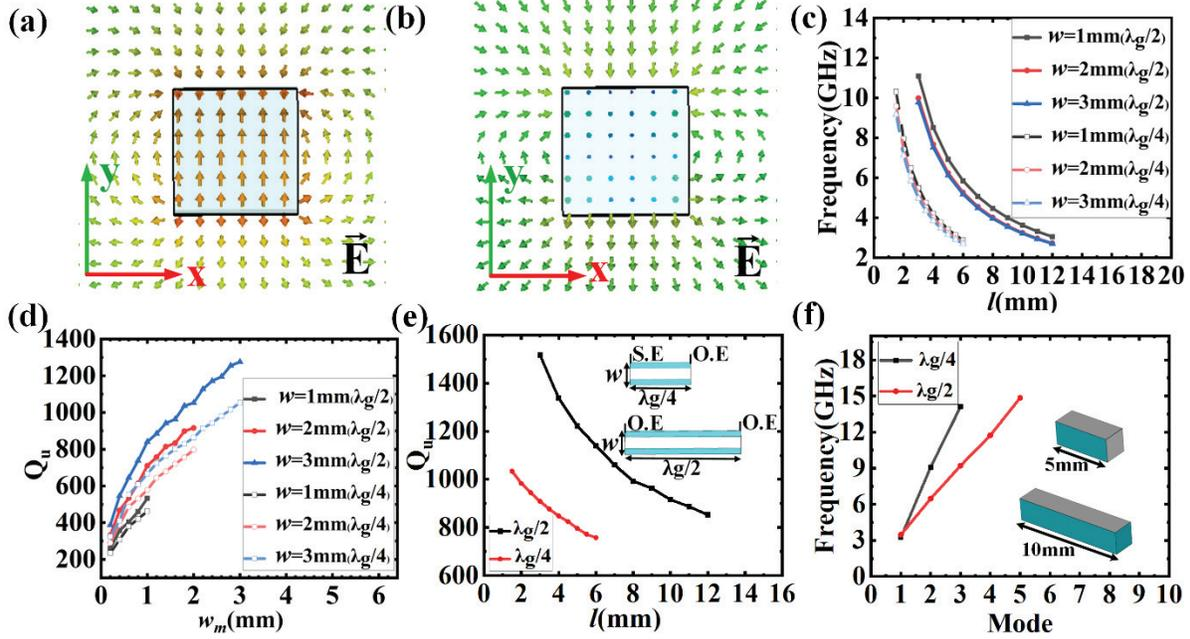
Fig. 2. (a) and (b) Electric field line distributions at the open and shorted end respectively. (c) Evolution of the resonance frequencies of ELSPRs with different  $l$  and  $w$ . (d) Evolution of  $Q_u$  with the variation  $w_m$ . (e) Evolution of  $Q_u$  with the variation  $l$ . (f) Evolution of the resonance frequencies of the  $\frac{\lambda_g}{4}$  and  $\frac{\lambda_g}{2}$  planar ELSPRs with mode number.
