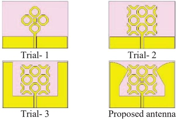
Fig. 1. Evolution stages for designing the proposed antenna.
