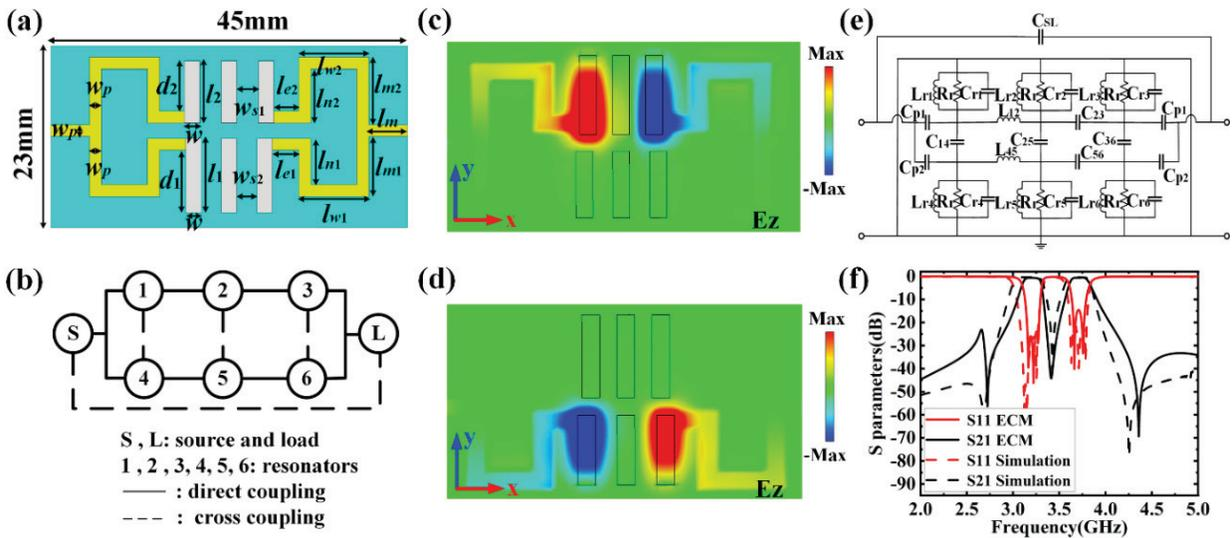
Fig. 4. (a) Layout of the proposed DBPF based on  $\frac{\lambda_g}{4}$  ELSPR. (b) Coupling routes. (c) and (d) Distributions of the electric field z-component at the center frequency of 3.1GHz and 3.6GHz respectively. (e) ECM of the proposed DBPF. (f) S-parameters comparison between the ECM simulation in Advanced Design System and CST simulations.
