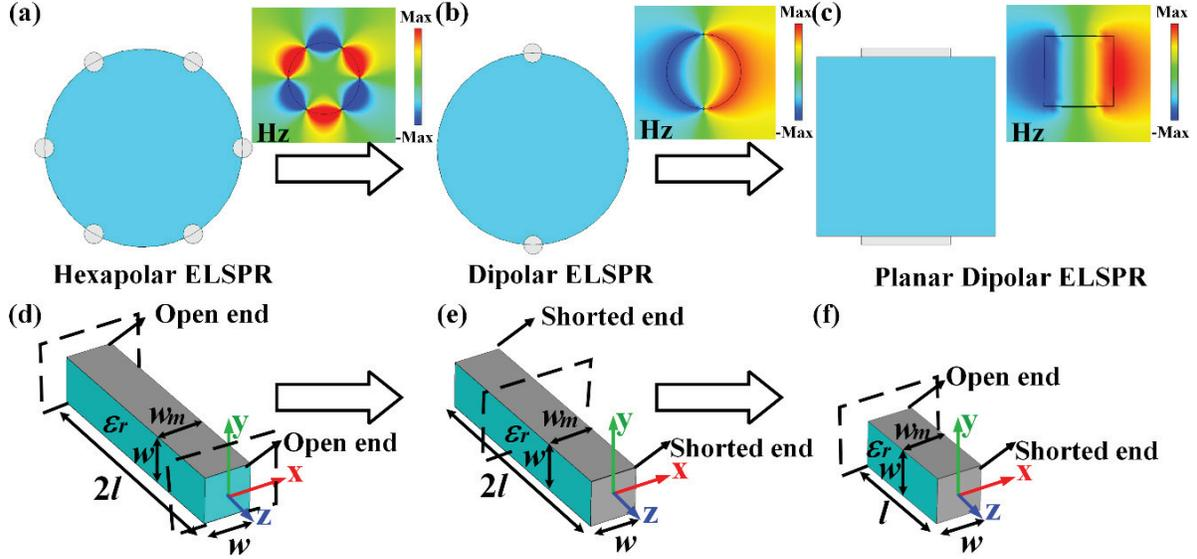
Fig. 1. (a-c) Cross-sectional view and magnetic field distribution of the hexapolar ELSPR, dipolar ELSPR, and planar dipolar ELSPR respectively. (d) A simplified ELSPR with open circuits at both ends. (e) A simplified ELSPR with short circuits at both ends. (f) A  $\frac{\lambda_g}{4}$  planar ELSPR with a short circuit at one end and an open circuit at the other end. The ‘blue’ region denotes the dielectric substrate and the ‘grey’ part denotes the metal patch.
