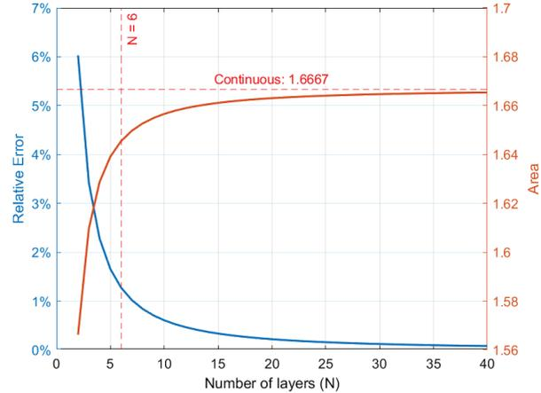
Fig. 12. Area under discrete LL permittivity distribution and the relative error versus the number of layers  $N$ .
