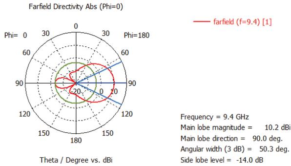
Fig. 13. The XZ plane of the radiation pattern.
