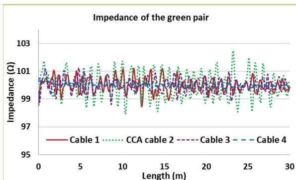
Fig. 3. Impedance profile of the green pair.
