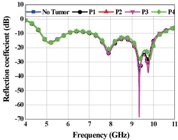
Fig. 19. The reflection coefficients  $S_{33}$  for all cases.
