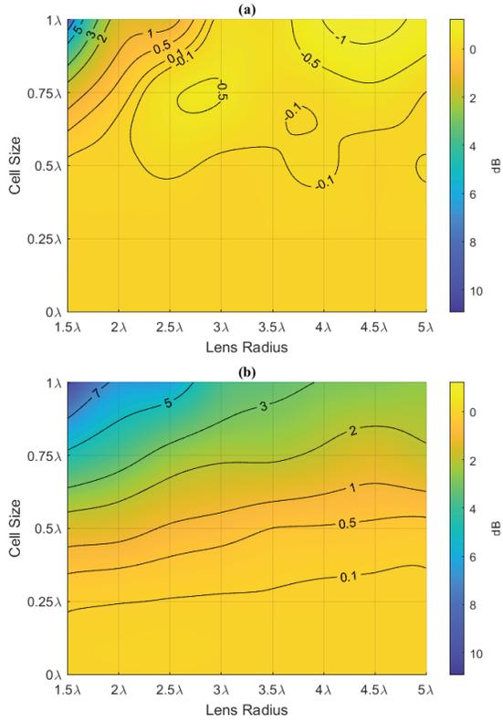
Fig. 17. Loss in RSSL due to quantization: (a) best case, and in (b) worst case. Best case includes areas where loss is negative. This means that the best case RSSL in these areas is better than the continuous counterpart lens.
