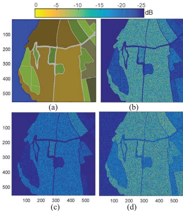
Fig. 5. Simulation of three-channel PolSAR image for the land region in Luxor city, (a) Ground-truth image showing the land type with indication of the soil water content, (b)  $|S_{hh}|$ , (c)  $|S_{hv}|$ , (d)  $|S_{vv}|$ , channels.
