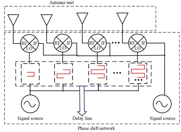
Fig. 2. Phase-shifting network structure based on delay line.
