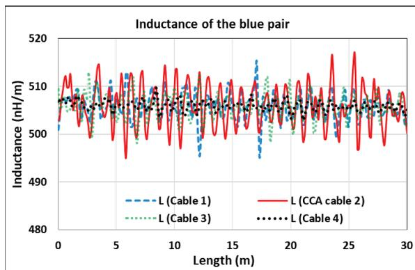
Fig. 14. Inductance comparison of the four cables using the blue pair.
