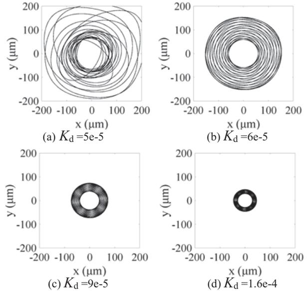
Fig. 17. Rotor orbit at 46 Hz for different  $K_d$ .
