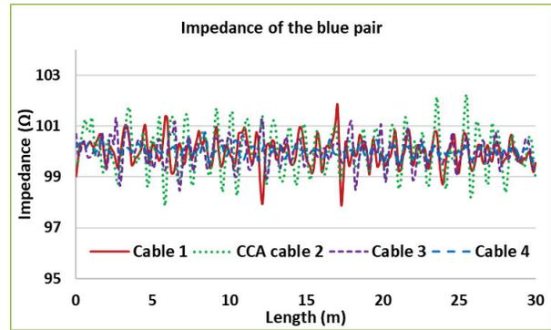
Fig. 4. Impedance profile of the blue pair.
