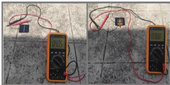
Fig. 10. Measurement of V<sub>OC</sub> and I<sub>SC</sub> of the solar cell with and without antenna integration.
