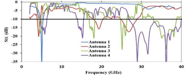
Fig. 4.  $S_{11}$  characteristics during the evolution steps.
