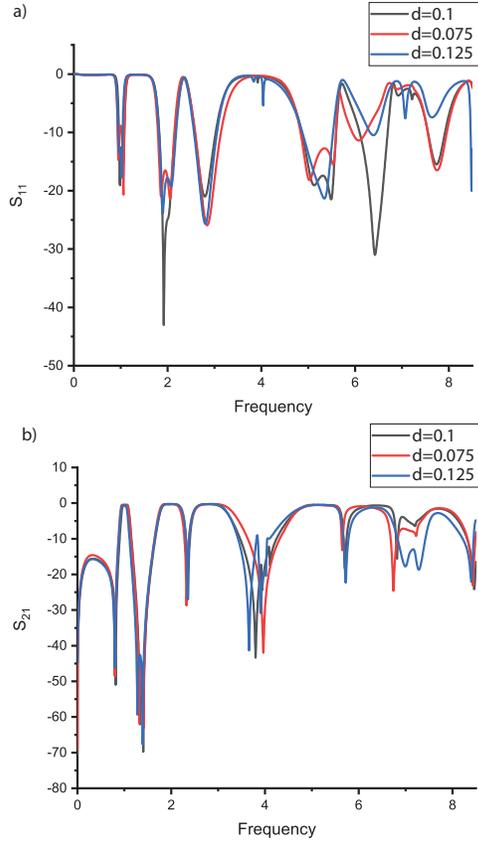
Fig. 5. The simulated S-parameters ( $S_{11}$  and  $S_{21}$ ) of coupling gap.
