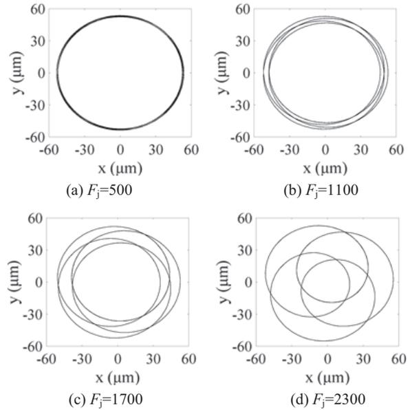
Fig. 21. Rotor orbit at 80 Hz for different  $F_j$ .
