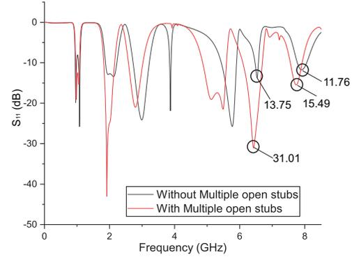
Fig. 4. The simulated  $S_{11}$  of the quad-section SIRs and loaded multiple stubs.
