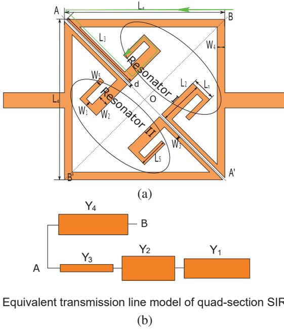
Fig. 1. Schematic of quad-section SIRs and equivalent circuit of quad-section SIRs. (a) quad-section SIRs. (b) Equivalent transmission line model of quad-section SIRs.
