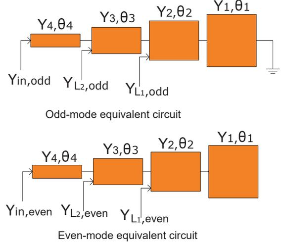
Fig. 2. Basic odd- and even-mode equivalent circuit of quad-section SIRs.
