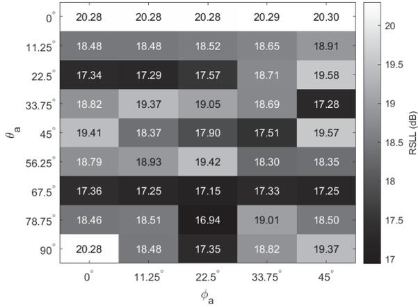
Fig. 13. RSLL matrix for the  $(\theta_a, \phi_a)$  sweep of lens ( $Q = 1\lambda, r_l = 5\lambda$ ). The spread in RSLL is 3.36 dB, however, there are multiple values that are better than that of the continuous reference.
