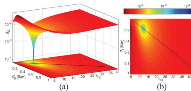
Fig. 7. Estimation of soil parameters for the grassland region named “Grass1”. Plots of the function  $\delta_G$  given by (15) versus the real dielectric constant  $\epsilon_{rg}$  and conductivity  $\sigma_g$  of a clayey soil; (a) 3D, (b) 2D, plot.
