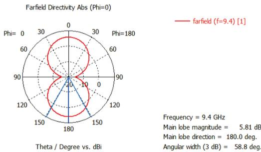
Fig. 7. The XZ plane of the radiation pattern.
