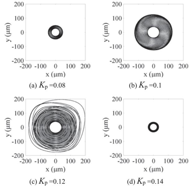
Fig. 13. Rotor orbit at 51 Hz for different  $K_p$ .
