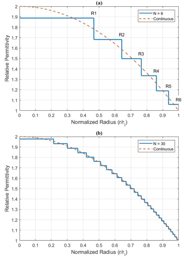
Fig. 10. Optimum layer relative permittivity  $\epsilon_n$  versus normalized radius  $r/r_l$  for  $N = 6$  in (a) and for  $N = 30$  in (b). The layer radii  $R1$  to  $R6$  in (a) correspond to similarly marked layers in Fig. 9.
