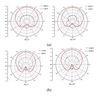
Fig. 11. The radiation patterns for the proposed CP filtering antenna: (a) Right-handed CP filtering antenna and (b) left-handed CP filtering antenna.
