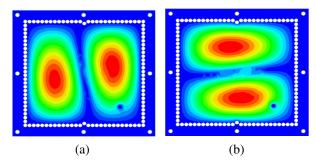
Fig. 3. E-field distributions of the bottom square cavity: (a)  $TE_{102}$  mode and (b) $TE_{201}$  mode.
