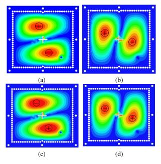
Fig. 4. Electric field distributions within one period for middle metal layer: (a) t = 0, (b) t = T/4, (c) t = T/2, and (d) t = 3T/4.
