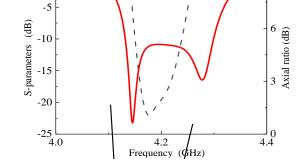
Fig. 9. The reflection coefficient and AR of the proposed left-handed CP filtering antenna.
